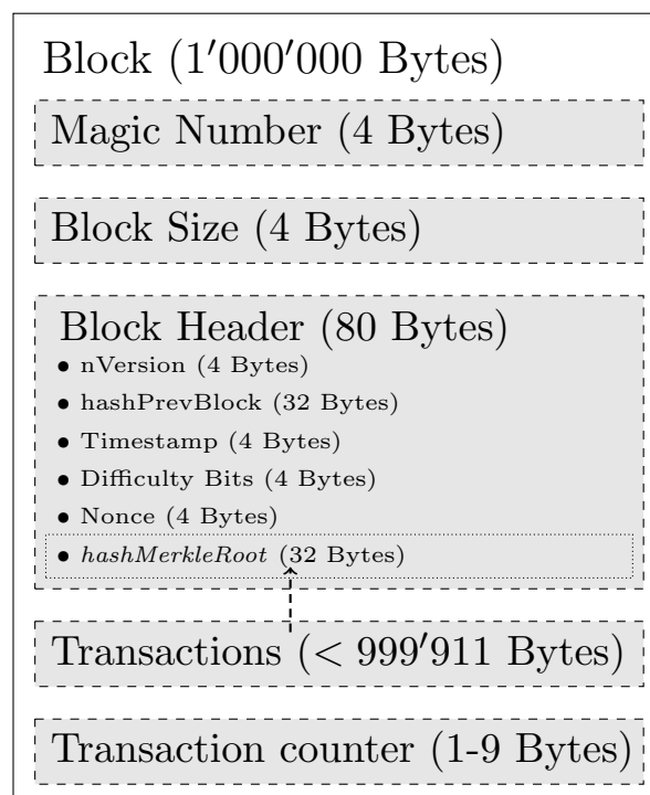
Figure 7: Structure of a block. [9] Note: The numbers in brackets show the size of the respective fields.
